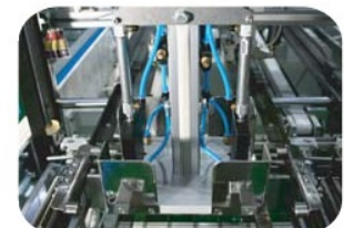
Forming head equipped with pneumatic pusher for easy carton uploading
