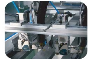
Pressurized hotmelt glue system
