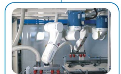
Double pick & place robots with vacuum pad pick up system
