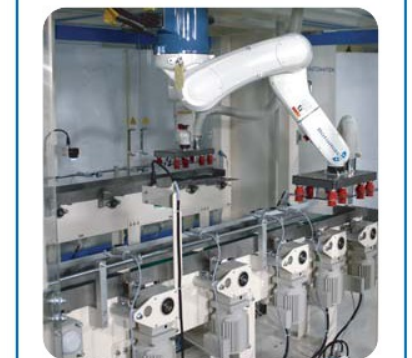
Multiple servo driven product feeding belt conveyors for product pitch control
